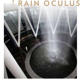
The *Rain Oculus*, another piece by Ned Kahn, collects and recycles rainwater which is used to fill the canal at The Shoppes and for bathroom flushing at the ArtScience Museum.
