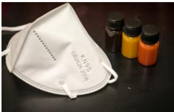
An KN95 certified mask made with dielectric nanofibre fabric alongside bottles of copper nanoparticles that add antimicrobial properties, Courtesy of Nanyang Technological University, Singapore.
